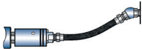
Hose should be a minimum of 300 mm long.
